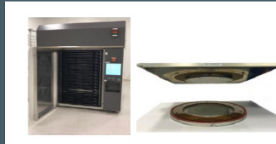
Figure 13: Burn-in process required to address early failures
